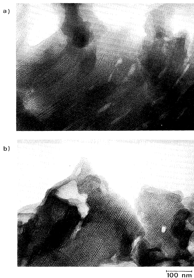
Fig. 6. Transmission electron micrographs of the a) octadecyltrimethylammonium-kanemite complex and b) calcined ( 700^\circ\text{C} ) octadecyltrimethylammonium-kanemite complex.
